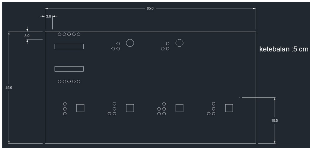
Rajah 1: Lakaran Single Phase Wiring Kit in Briefcase
