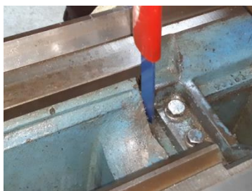
Figure 4.3 Iron plate able to reach small and narrow gap of machine
