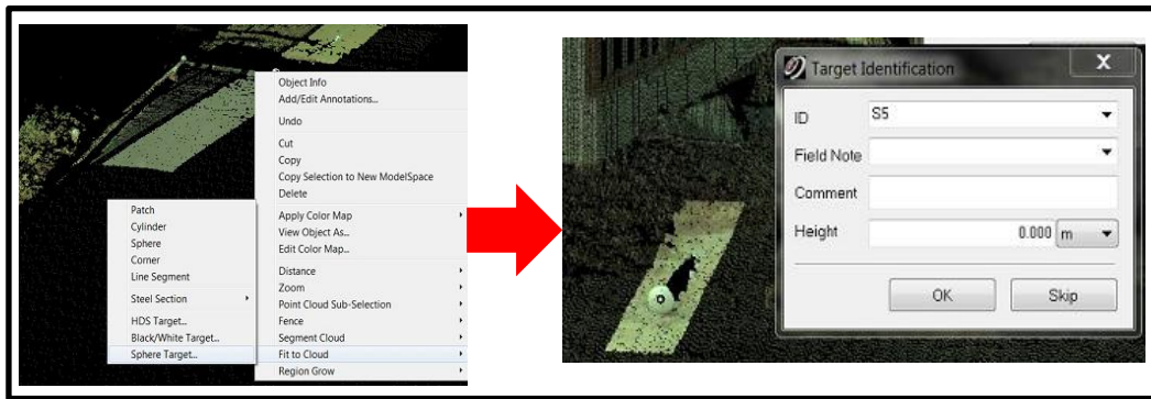
Figure 7: The registration process using spherical target for 2 scanning station.
