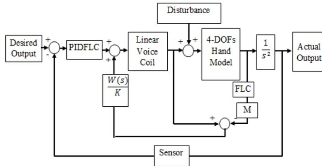
**Figure 1** Schematic diagram of proposed control scheme
