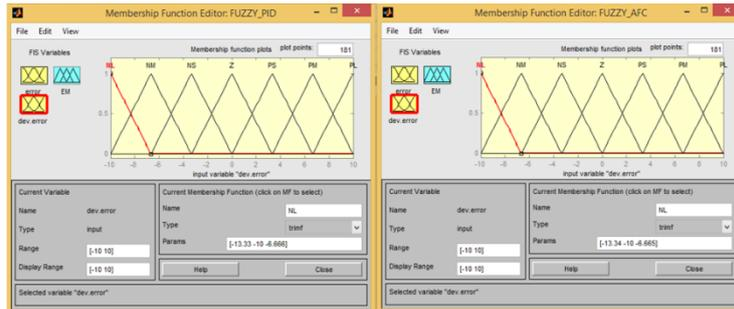
Figure 4 Triangle shaped membership functions command window of derivative error for PID and AFC controller (range in [-10 10])
