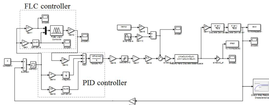
Figure 7 4-DOFs Simulink modelling controller system using adaptive PIDFLC
