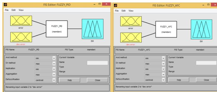
**Figure 2** Fuzzy Logic toolbox command window with two inputs and one output for PID and AFC controller.
