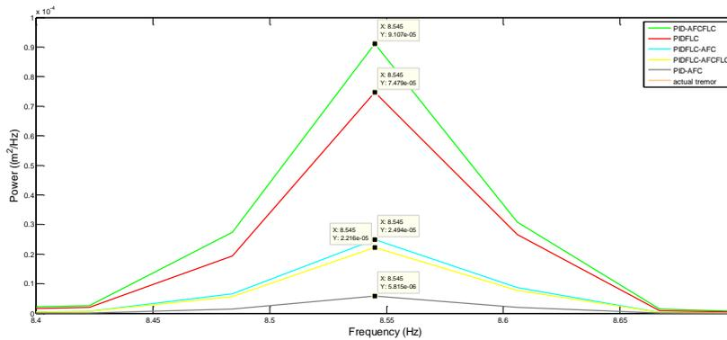
**Figure 16** Comparison the PSD  $((m / s^2)^2 / Hz)$  against displacement frequency (Hz) between the five control models, (PIDFLC, PID-AFC, PIDFLC-AFC, PID-AFCFLC and PIDFLC-AFCFLC) and actual displacement of PD patients. (Zoom mode)
