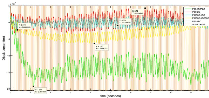
**Figure 14** Comparison between five proposed control models (PIDFLC, PID-AFC, PIDFLC-AFC, PID-AFCFLC, PIDFLC-AFCFLC), and actual displacement of PD patients. (Zoom Mode)
