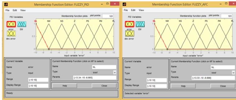
Figure 3 Triangle shaped membership functions command window of error input for PID and AFC controller (range in [-10 10])
