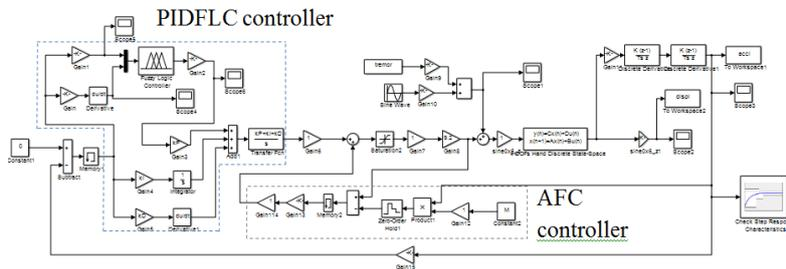
**Figure 10** 4-DOFs Simulink modelling controller system using adaptive hybrid PIDFLC-AFC
