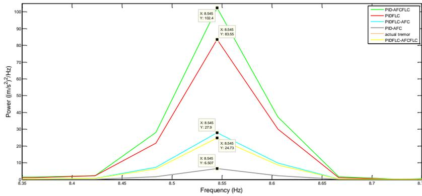
**Figure 20** Comparison between the PSD  $((m / s^2)^2 / Hz)$  against acceleration frequency (Hz) for five control models (PIDFLC, PID-AFC, PIDFLC-AFC, PID-AFCFLC and PIDFLC-AFCFLC) and actual acceleration of PD patients. (Zoom mode)
