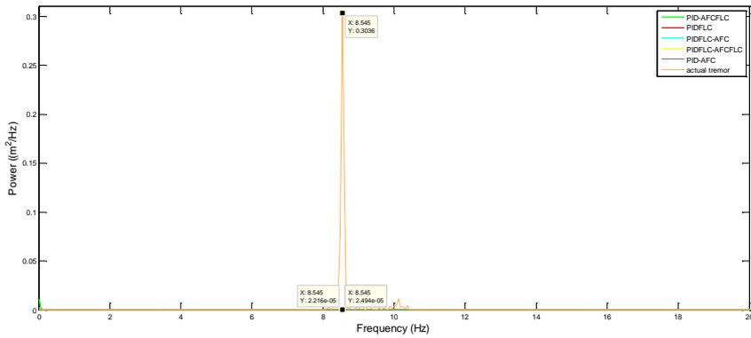
**Figure 15** Comparison the PSD  $((m / s^2)^2 / Hz)$  against displacement frequency (Hz) between five control models, (PIDFLC, PID-AFC, PIDFLC-AFC, PID-AFCFLC and PIDFLC-AFCFLC) and actual displacement of PD patients.
