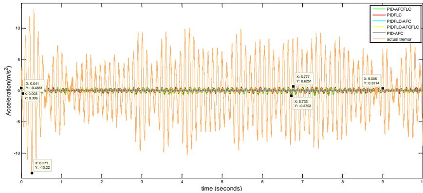
**Figure 17** Comparison between five proposed controller models (PIDFLC, PID-AFC, PIDFLC-AFC, PID-AFCFLC and PIDFLC-AFCFLC) and actual acceleration of PD patients
