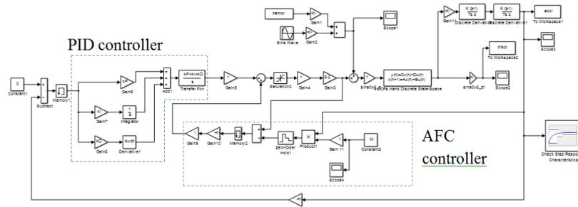
**Figure 8** 4-DOFs Simulink modelling controller system using hybrid PID-AFC
