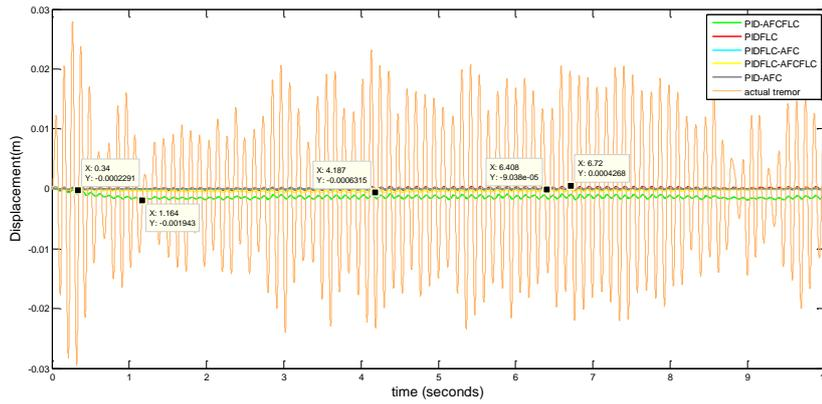
**Figure 13** Comparison between five proposed controller models (PIDFLC, PID-AFC, PIDFLC-AFC, PID-AFCFLC, PIDFLC-AFCFLC), and actual displacement of PD patients.
