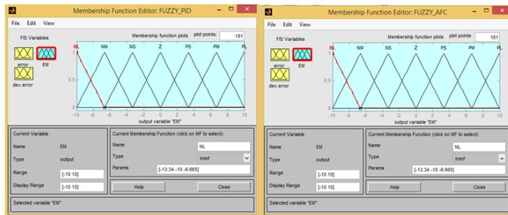
Figure 5 Triangle shaped membership functions command window of output, EM for PID and AFC controller (range in [-10 10])
