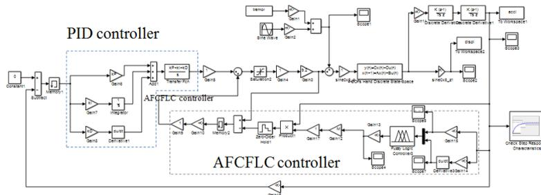
**Figure 9** 4-DOFs Simulink modelling system using adaptive hybrid PID-AFCFLC
