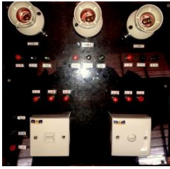
Two Way Switch Assembly
