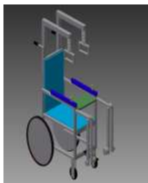
Figure 1: Auto CAD Drawing of 10 in 1 Physiotherapy Wheelchair
