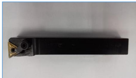
Figure 2: Tungsten Carbide Cutting Tool
