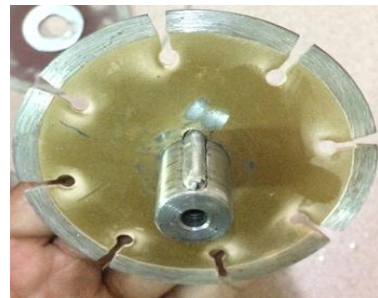
Figure 5b Modified Concrete Cutter Disc Diagram
