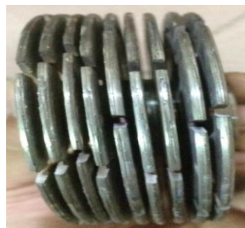
Figure 7 Concrete Cutter Discs and Steel Flat Washers Arrangement Diagram
