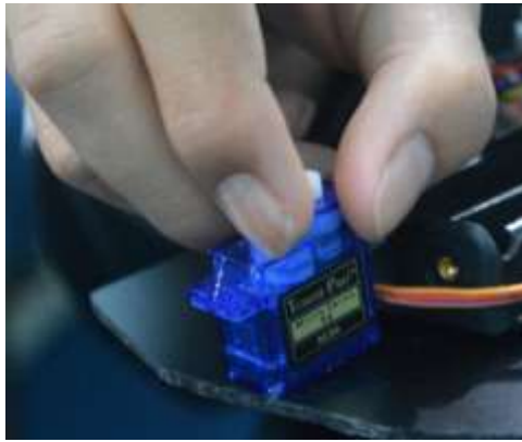
Figure 10 Motor Servo Installation
