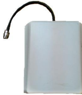
Figure 2.2: patch antenna with plastic Radom cover
