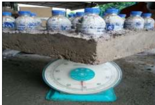
Figure 3. Concrete block masonry are weighed before soaked in the water
