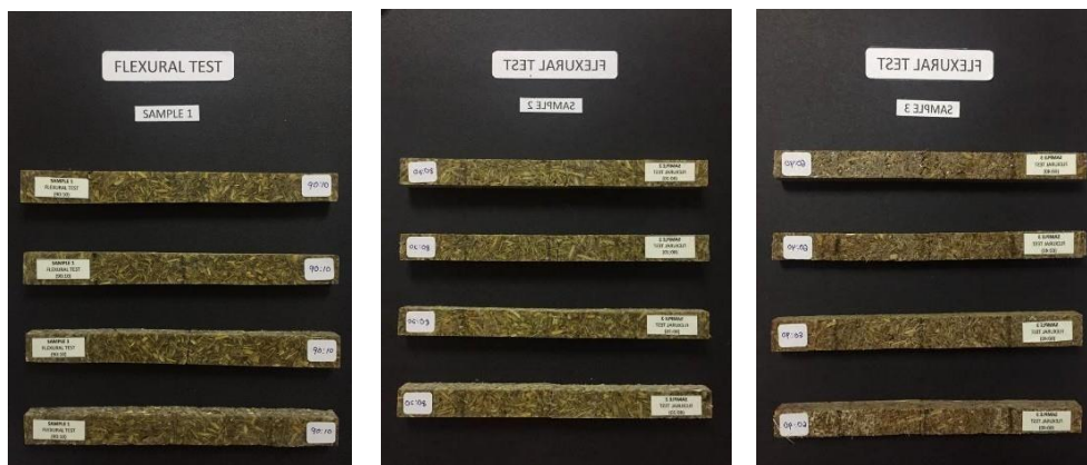
Figure 4.2.1 Sample After Flexural Test Performed
