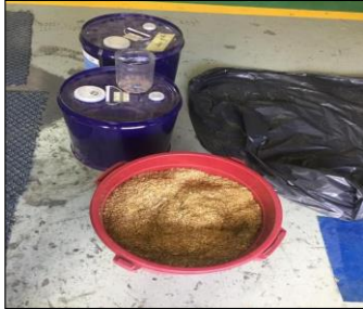
Figure 3.3.1 Paddy Straw and Epoxy
