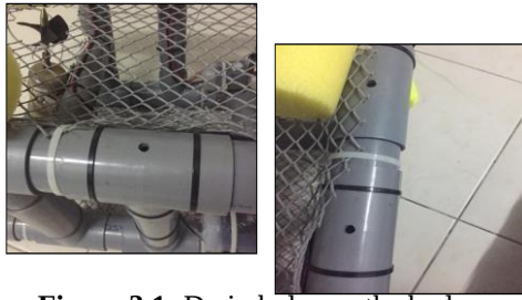
Figure 3.1: Drain holes on the body
