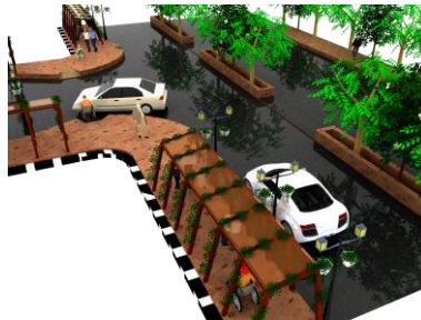
Figure 27 : New pedestrian design to disable person with curb ramps curb extension ,signaling, handrail ,signal ,and handicapped parking.
