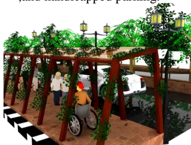
Figure 27 : New pedestrian design to disable person with curb ramps curb extension ,signaling, handrail ,signal ,and handicapped parking.
