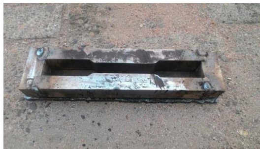
Figure 7 Composite moulding process according to ASTM Standard D 638 -III
