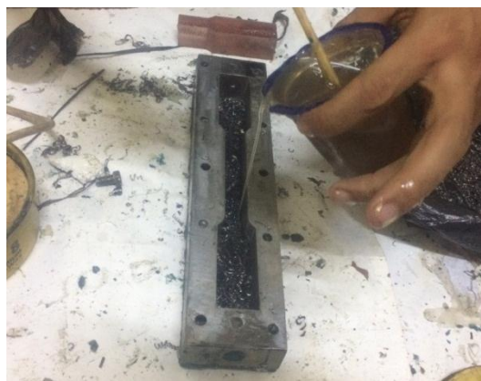
Figure 14 pouring of polyester + hardened into moulding
