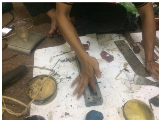
Figure 12 lubricating the lubrication so that the mould wall is not sticky with the specimen
