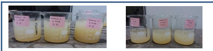
Figure 3.2 : water sample of 0.5g and 1.0g dosages of MO seeds powder
