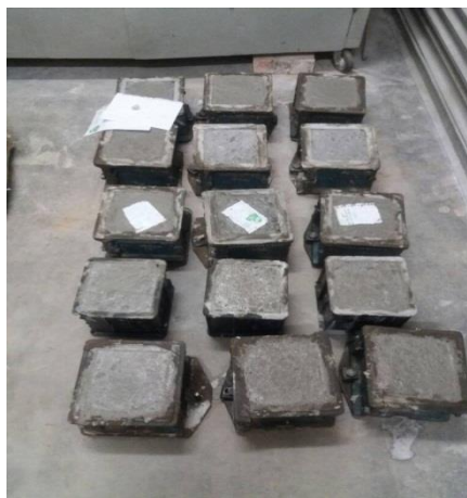
Figure 5 Concrete Cube Test
