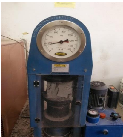
Figure 6 Compressive Strength Test
