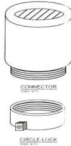
Figure 5: The screw method is used to attach the connector to the circle lock.
