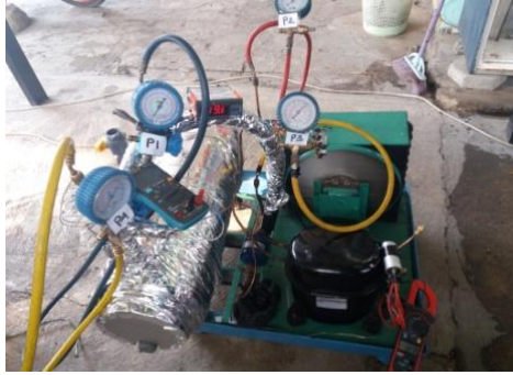
Figure 11. Water Cooling Machine Unit
