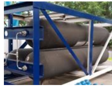
Figure 6. CNG gas cylinders filled with 200 Nm 3 of gas
