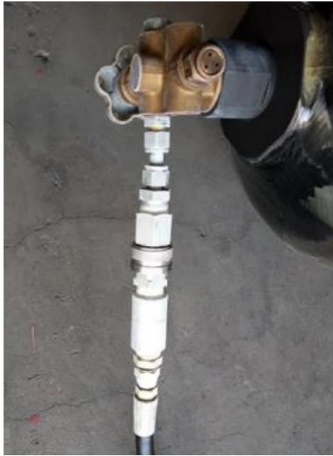
Figure 16. Example of a photo of the observation of the Joule Thomson Effect phenomenon that occurs when gas flows from a Cylinder CNG with a pressure of 250 BAR to PRS.
