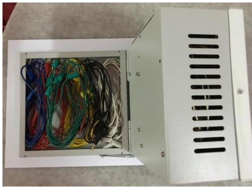
i. Front view of cable storage space
