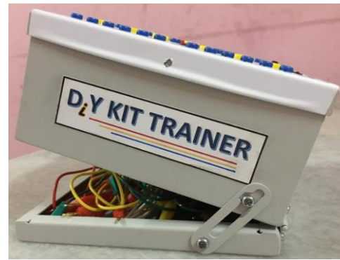
ii. Side view of cable storage
