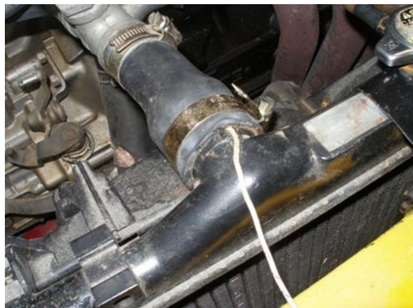
Figure 3 Three K-type thermocouples were used to measure temperature at various points on the radiator to log the temperature.
