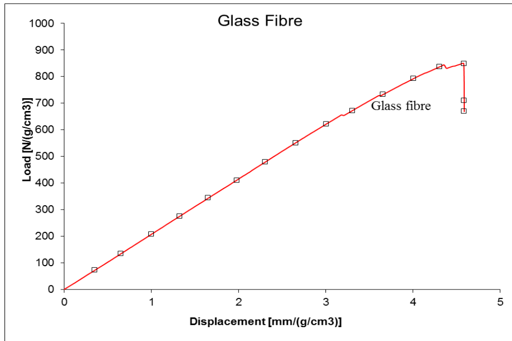
Figure 2 : Load-Displacement Extension Curve Under Compression
