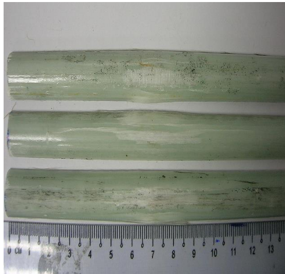
Figure 5: Failure Mode for Glass Fibre Reinforced Composites under Flexural Loading
