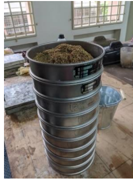
Figure 2.4.2 The sample was placed into nine stage of the sieve of a Nest of ISO
