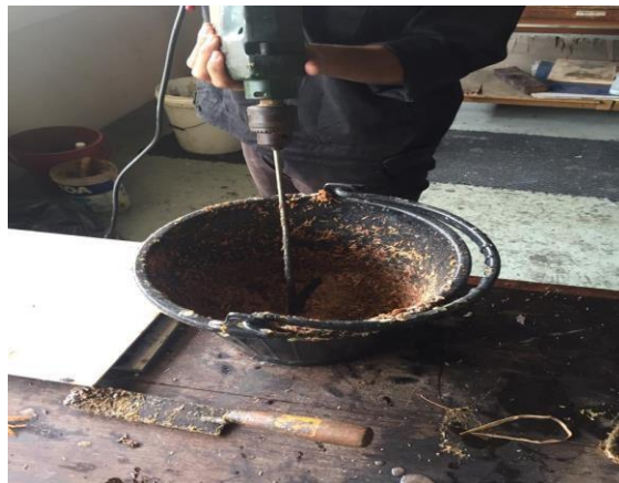
Figure 2.2.1 The fibers and resin were mixed by hand drill mixer
