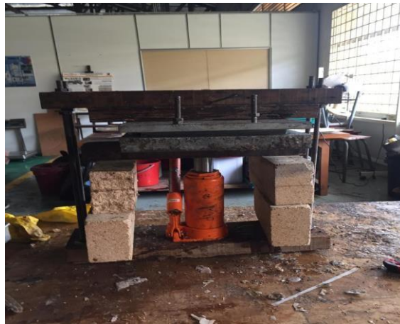
Figure 2.2.2 Mixtures were put into the mould and pressed
