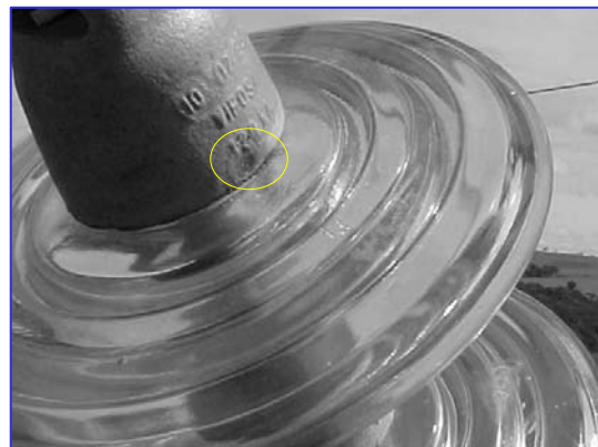
Fig. 3 – Damage due to destructive effect of current flow through the insulator following a backflashover (a corrosion process was initiated after the damage)
