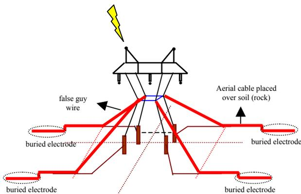
**Figure 3 – False guy wires configuration**
