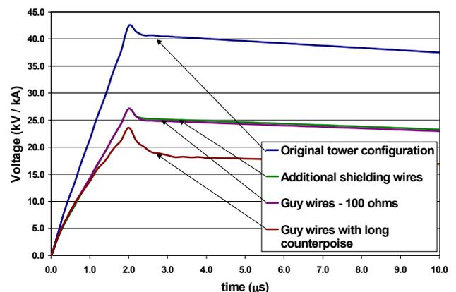
Figure 2 - Developed overvoltage across insulator string
