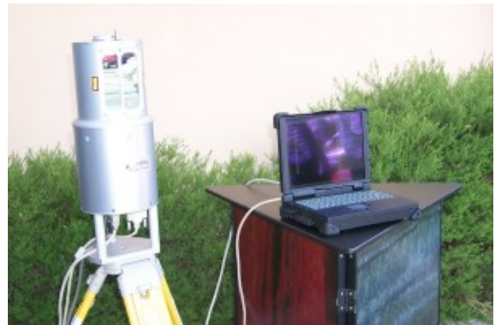
the field - the laser scanner (left) and a laptop (right).
