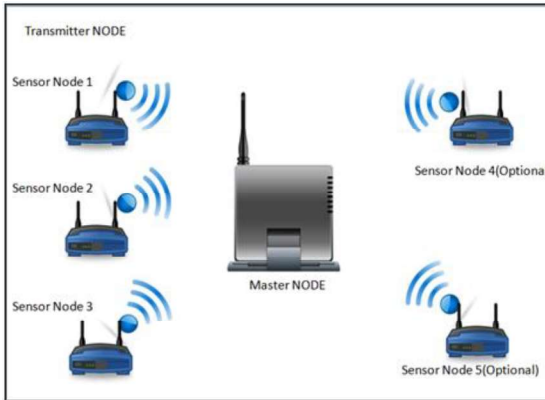
Fig. 2 Stat Topology of sensor network
