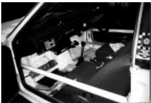
PICTURE ABOVE: Lots of goodies in this pic, like the side rollbars and the Halda positioned in the glovebox to mention a few things.
