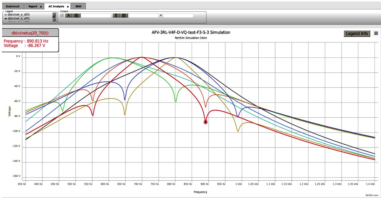
\*\*\* At 900 Hz, the **Red Dot on Notch** indicates **-86 dB attenuation** for the **f(700)** trace .
