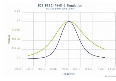
Resulting signal level of K = -28 dB at 1000 Hz. Results depend on amount of Dual-Channel Spread. No precision components required. Caps are +/- 5%, f() is corrected by the MFB circuit at R(freq) for each stage.
