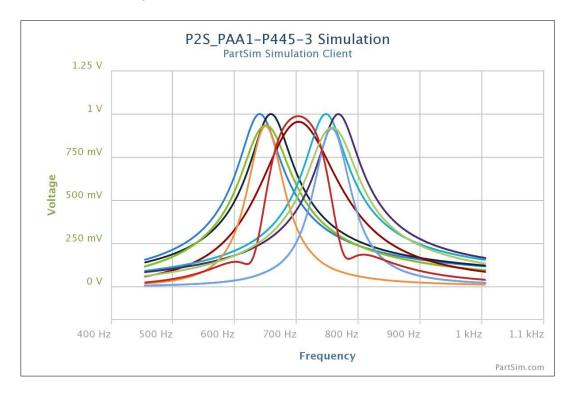
The Dark-Red trace is the broader original CW signal The Light-Red trace is the narrow Double-Notched PassBand Signal.
