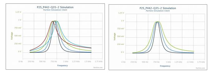
Top = 65Hz \_\_ at -1dB and BW = 110 \_\_ at -3dB Variance = 14 Hz per dB attenuation \_\_ Last Stage Filter: measured "Q" = 6.5 \_\_max Chapter: AFX\_rFilter\_5\_P2S  $_{210801}$  4/20
