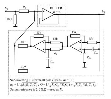
**Fig.2**. Realization by means of buffer and noninverting FBP; ",3 x 741"; supply  $U_{CC} = \pm 15$  V;  $R_a = 122k$ ;  $R_m = R_n = 1k3$ ; C = 10 nF: measured  $f_0 = 11$  kHz;  $Q_e = 27$ , 5; for U<sub>1</sub>less than 4 V (for larger amplitudes take effect slew rate)
