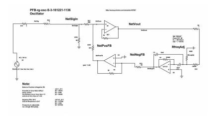
\*\*\*\*\* Positive Feed-Back with limiter control \*\*\*\*\* produces a "SINE" V(out) , with single resistor f() control.
