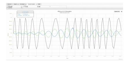
V(out) is NetVout f(0) = 700 Hz FeedBack Q=2 Effecive Q=7 BW=100 Hz
