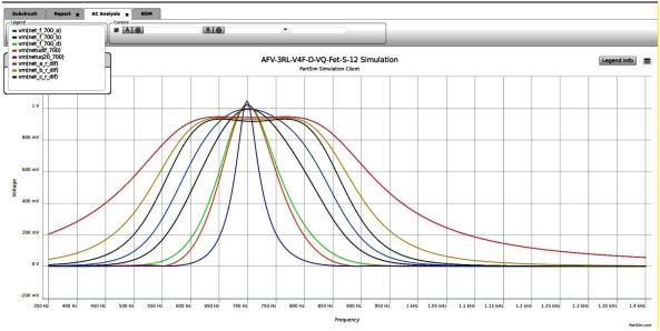
\*\*\*\* Below : shown adjusted 600Hz , 700Hz , 800Hz \*\*\*\*\* Notice that the peak amplitudes of the final signals stay within 0.3 dB of the f(700) signal.
