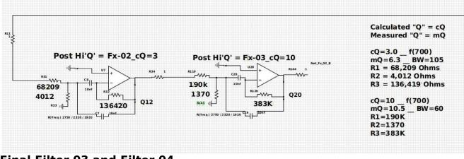
Final Filter 03 and Filter 04 are for producing an enhanced Narrow Band-Pass.
